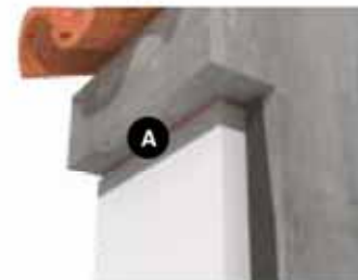
Details for applying joint base and Pumalastic® MS (A)
