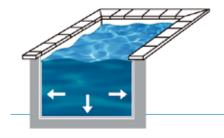
The ceramic tiles will have to withstand the large pressures generated by the water in the swimming pool as well as negative pressures when the pool is emptied for maintenance.
